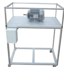
Three Phase Induction Motor : G-200410
