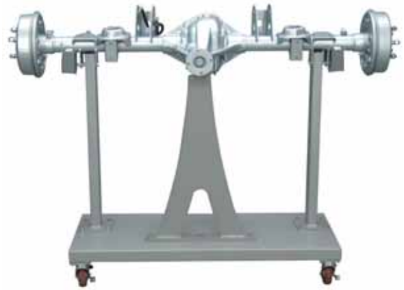
23-038 SUV, Rear Axle Exhibit Equipment Model No. G-3 SUV, 후차축 전시장비 G-230602
